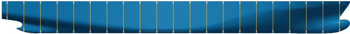
Figure 6. The surface of the DTC hull. The highlighted sections divide the ship into 20 equispaced chunks at the free-surface level.
