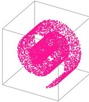
Figure 4.1: 2d Swiss Roll embedded in a 3d space. In this example the data lay on a surface that can be parametrized using two coordinates thus its intrinsic dimension is 2 while the embedding dimension is 3.
