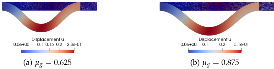
Figure 6.19: High fidelity displacement u for the SVK beam with B = (0, -1000) at \mu = 0.2 for different geometries.
