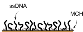
Fig. 2.16. Cross section of the mixed SAM formed by ssDNA- and MCH-molecules. MCH-molecules compete with unspecifically bound ssDNA-molecules, removing them and chemisorbing onto the surface through S-Au bond ( \approx 2 eV ).
