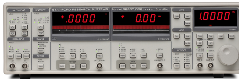
Fig. 2.10. Front panel of the lock-in amplifier, model SR830 by Stanford Research Systems.
