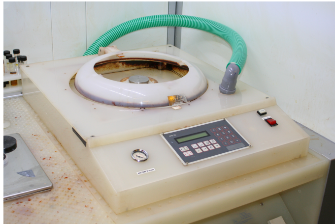
Fig. B.1. Picture of the spin-coater used during the thesis-work. Its main features are listed in Table B.1.
