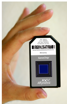
Figure 5.1: Example of an Affymetrix chip - Reproduction of a high-density oligonucleotide microarray often referred to as a chip. The small dimensions of the chip ( 1.28 \text{ cm}^2 ) are compared to a human hand. The image is courtesy of Affymetrix, Inc., Santa Clara, CA, USA.
