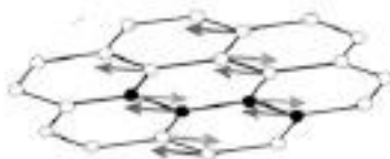
Figure 2. E_{2g} vibration mode of graphene.
